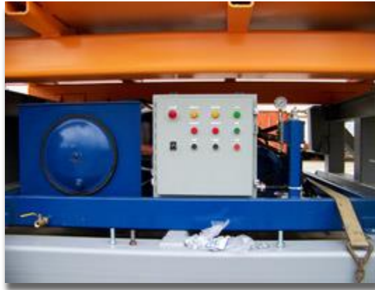
Hydraulic Drive Unit
